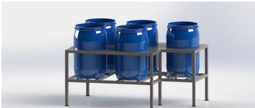
Gambar 2. Gambaran alat komposter parallel drum
